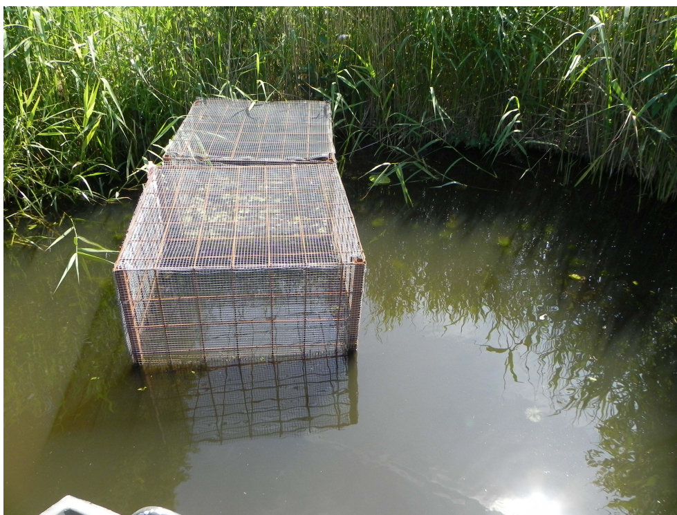
Figure 11. Two cages used to exclude the inflow of plant fragments.
